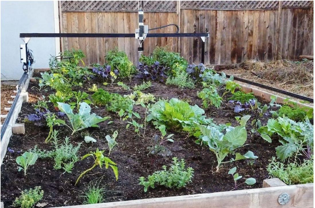
FarmBot is an open-source automated farming machine. Rory Aronson, the founder of the project writes: “Picture it as a giant 3D printer outfitted with a seed injector, sprayer, plow, and sensors.”
