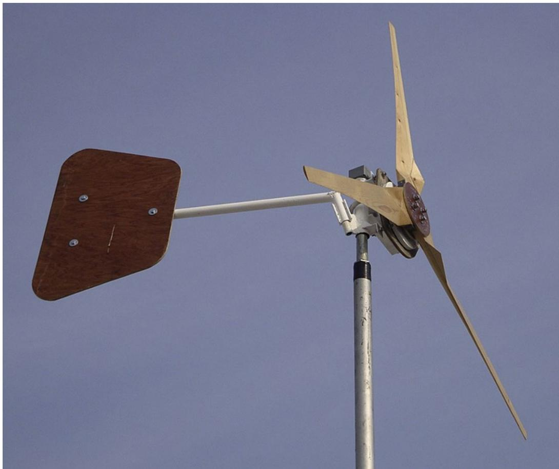
Fig. 2. A locally manufactured small wind turbine of rated power 600 W at 10 m/s, able to produce energy of 1270 kW h/year at a 5 m/s mean wind-speed location.
